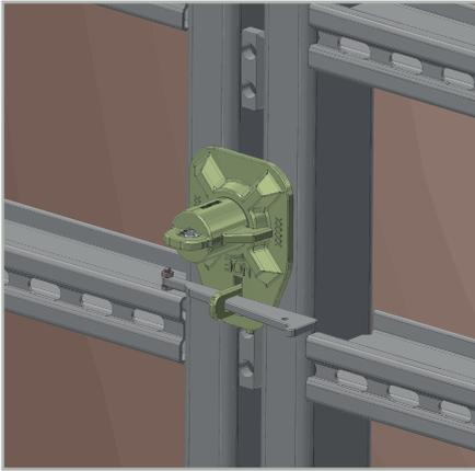
Install swivel bearing on first-face formwork
