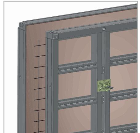
Insert tie rod and install the swivel plate with wing nut
